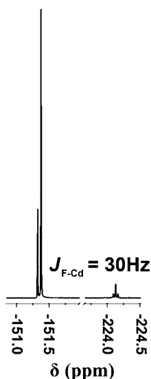
Figure 4. ^{19}\text{F} NMR spectrum of [\text{Cd}_2(\mu\text{-F})(\mu\text{-L}_m^*)_2](\text{BF}_4)_3 .
